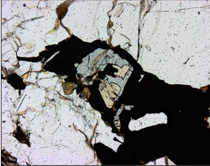
**Figure 74:** Grain of gahnite (bluish) with inclusions of partially resorbed staurolite (light brown). Sample from the Raudsandhaugtjern prospect no.4. The gahnite grain is about 300 microns across.
