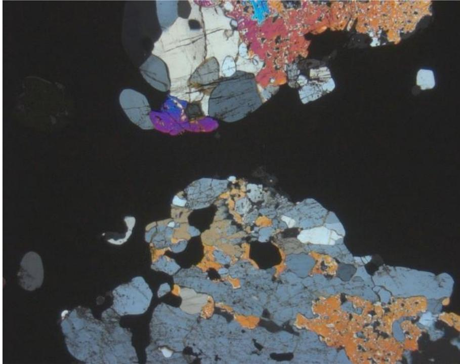
**Figure 78:** Photomicrograph from the Hellerfjellet deposit showing celsian (dark grey), quartz (light grey) and staurolite (colored) as matrix phases between sulfides (black).
