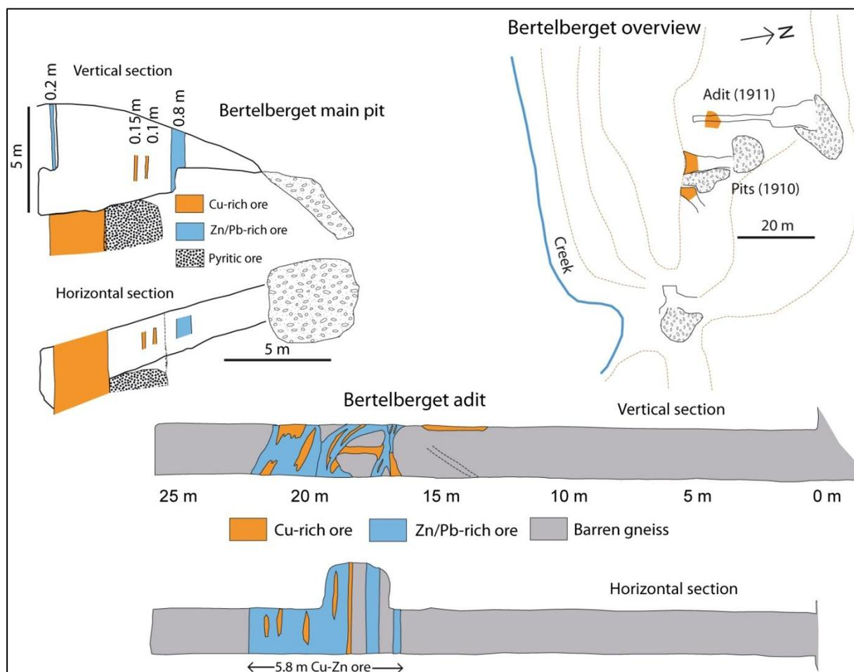
Figure 36: Plan view and detailed cross sections of main workings of the Bertelberget mine, showing the distribution of the different ore types (modified from Krefting, 1911).
