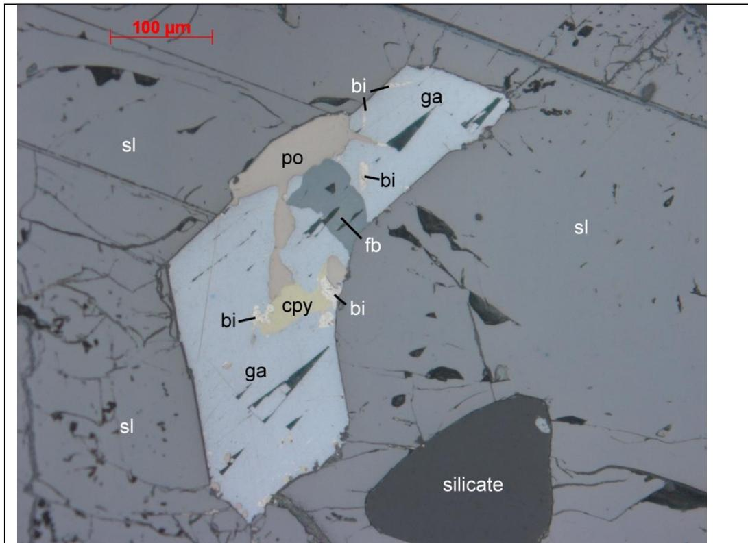
**Figure 82: Photomicrograph from the Skarbekken prospect, showing a grain of galena (ga) in sphalerite (sl), intergrown with pyrrhotite (po) and chalcopyrite (cpy) and with inclusions of freibergite (fb) and native bismuth (bi).**
