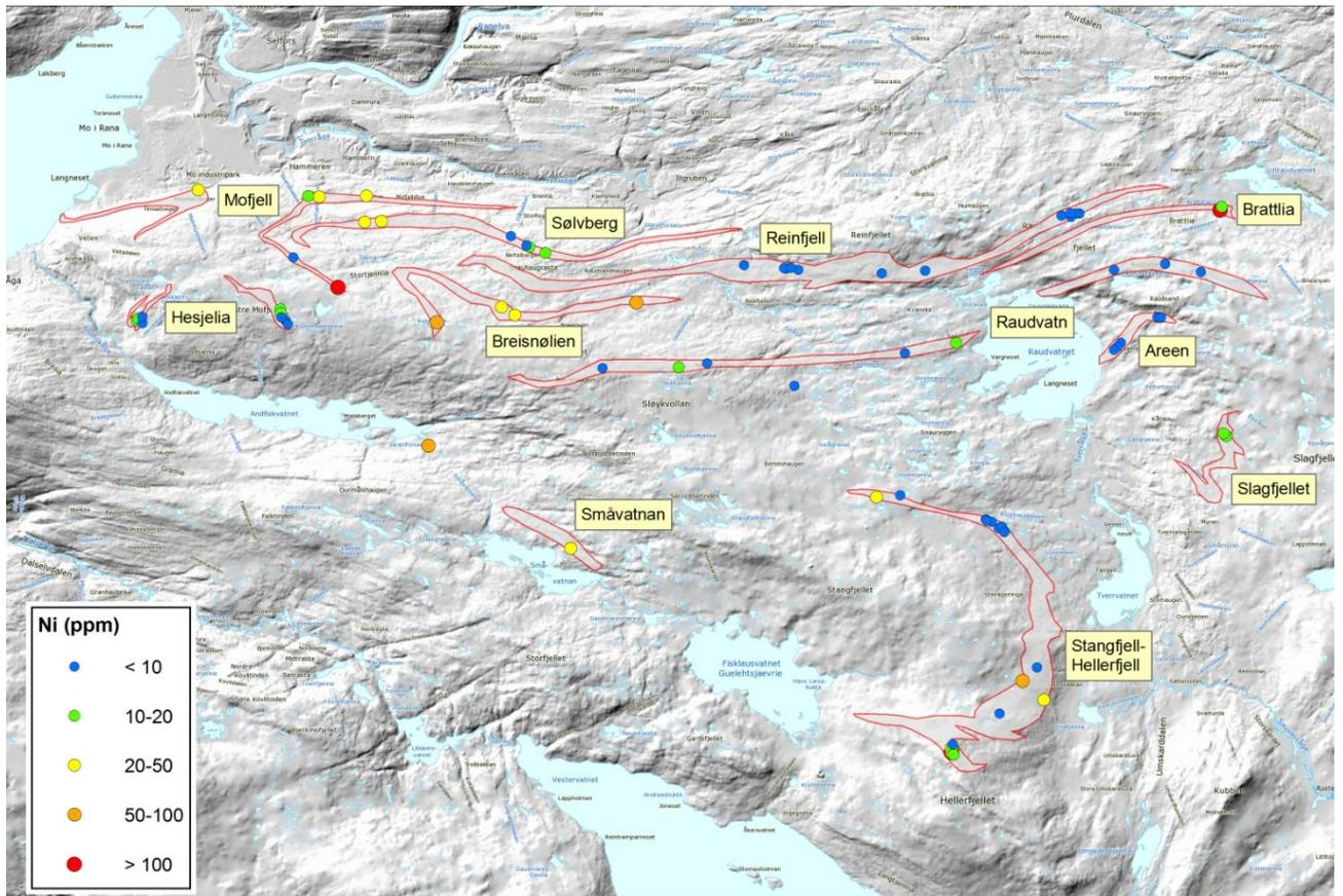
Figure 66: The zones of sulfide mineralization showing the average content of nickel in the main deposits.
