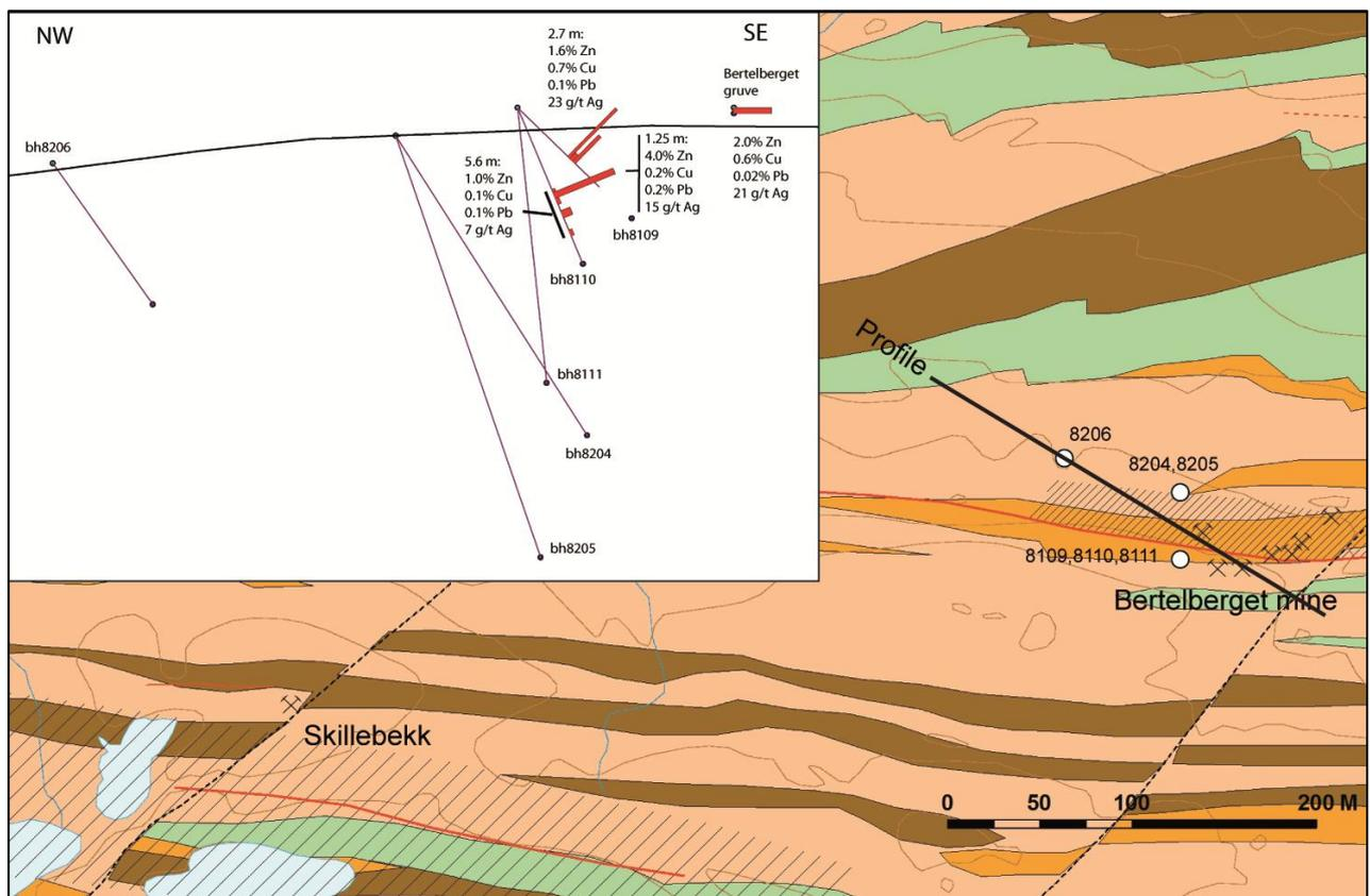
**Figure 35: A section of the map in Figure 32 and a vertical profile through the Bertelberget mineralization, showing projected drillholes with metal values. The superimposed hatched areas and red lines mark distinct geophysical conductors (TURAM, Dalsegg, 1984).**
