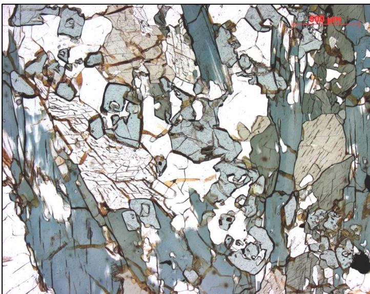
**Figure 76:** Grains of gahnite (light bluish prisms) overgrowing clinoamphibole (light to dark green). Sample from the Thermos main prospect.
