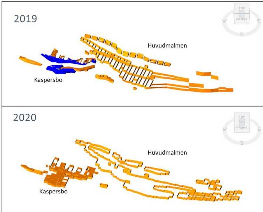
Figure 3-10. Example of changes in resource and reserve in Kaspersbo and Huvudmalmen at level -1040z.
