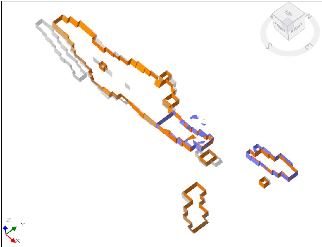
Figure 3-8. Oblique view of Kvarnberget level -730z. The outline of 2019 reserve is in grey, and the 2020 reserve is in orange. Several of the stopes were either shortened or discarded in the new design. The blue shape is the central pillar of Kvarnberget which was included in the reserve in 2020.
