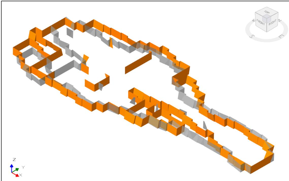
Figure 3-9. Oblique view of Lappberget level -1340z. The outline of 2019 reserve is in grey, and the 2020 reserve is in orange. In the new design, some of the stopes are wider on the edges, some new stopes were included on the western side of Lappberget.
