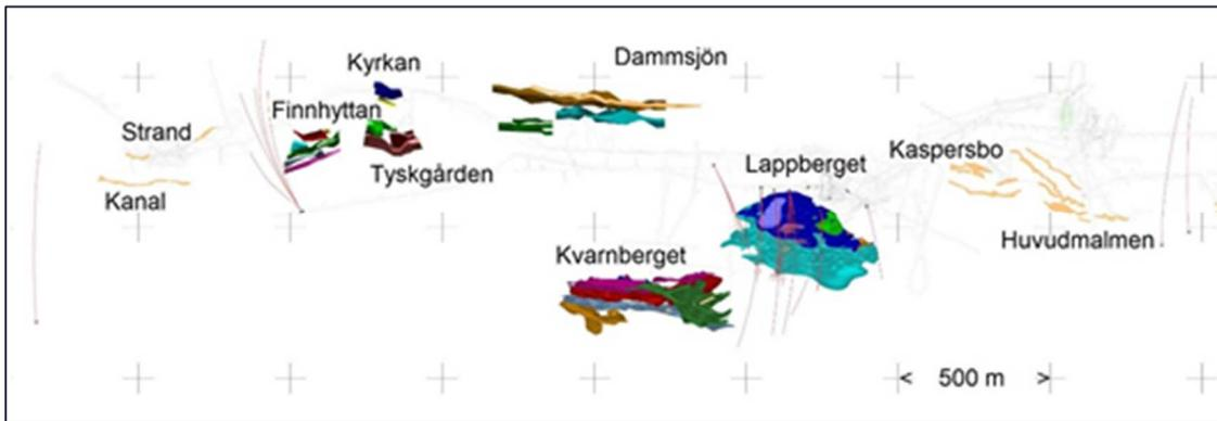
Figure 3-6. Distribution of near mine exploration resource drilling (red traces) in 2020.
