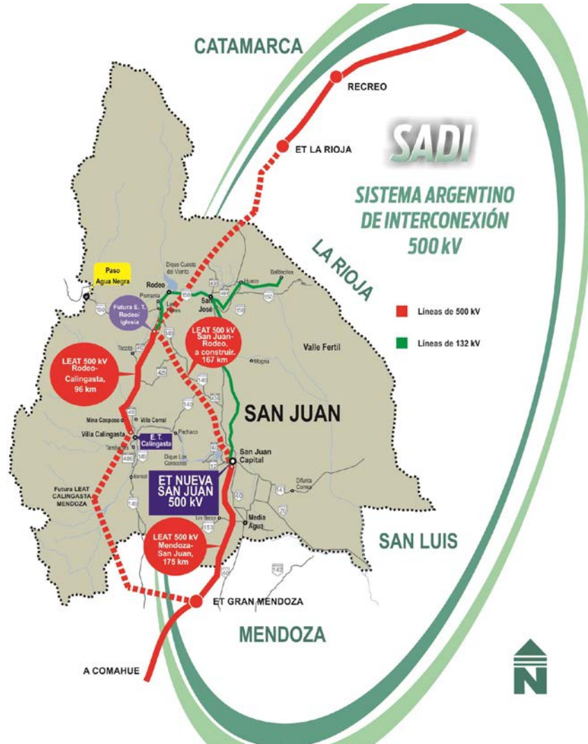
Figure 18-17: EPRE's vision for a 500 kV Interconnection Network for the Province of San Juan (extracted from June 2017 publication by EPRE)
