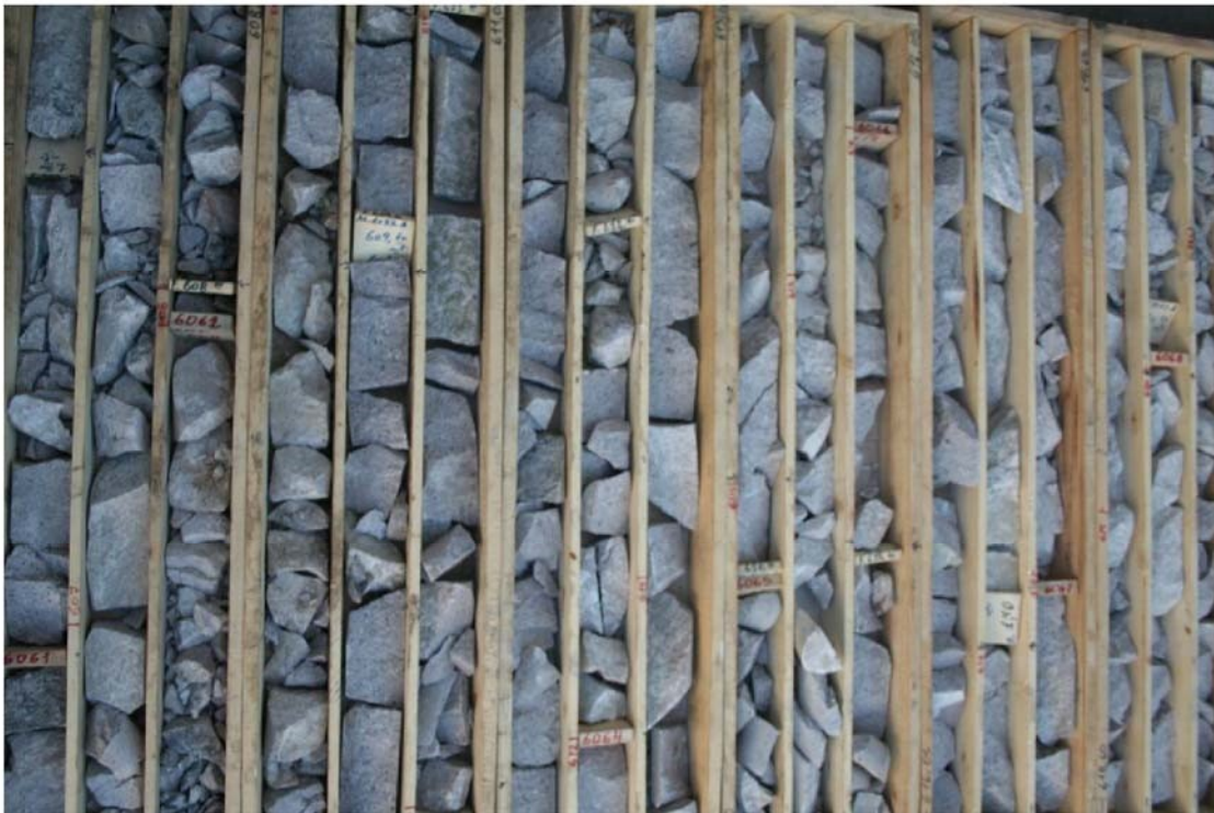
Figure 7-20: Typical Drill Core from Los Azules indicating the strongly fractured nature of the rock (Jemielita, 2010)
