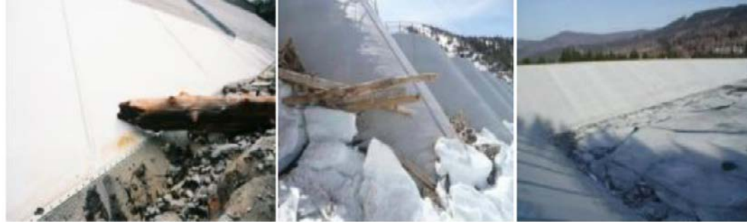
Figure 18-41: Examples of Resistance of Exposed SIBELON CNT PVC geocomposites to extreme cases of impact by debris/ice
