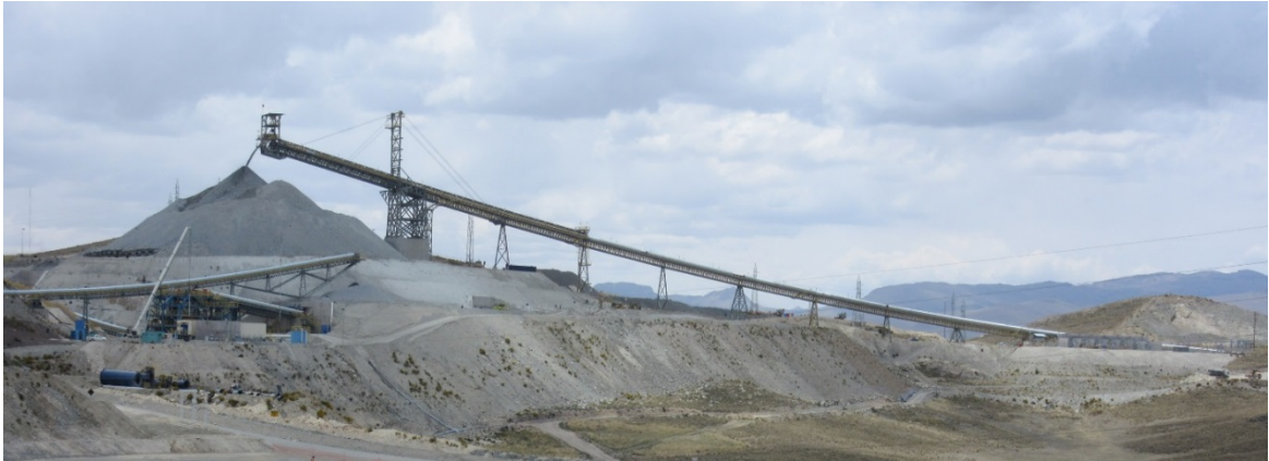
Figure 17-7: Photo of the coarse ore overland conveyor delivering coarse ore.
