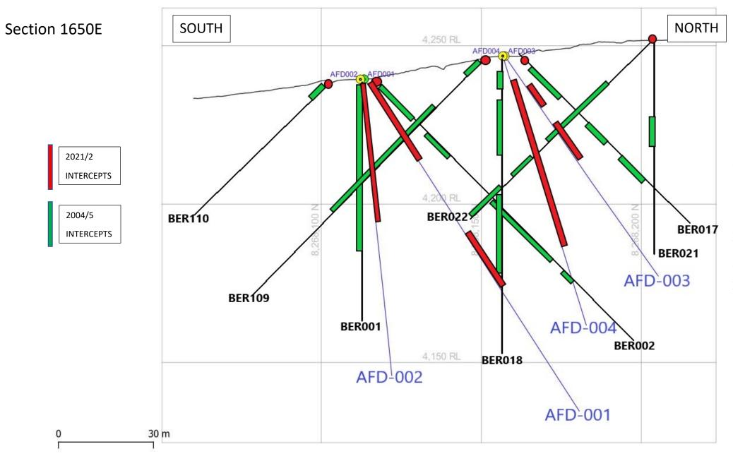
AFD holes are 2021/2 diamond drilling. BER holes are 2004/5 RC drilling.
