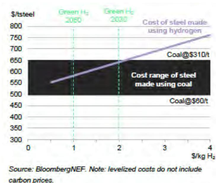
**Figure 31 – Levelized Cost of Steel Production**
