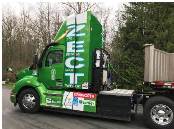
**Figure 24 – Fuel Cell Electric Drayage Truck**
