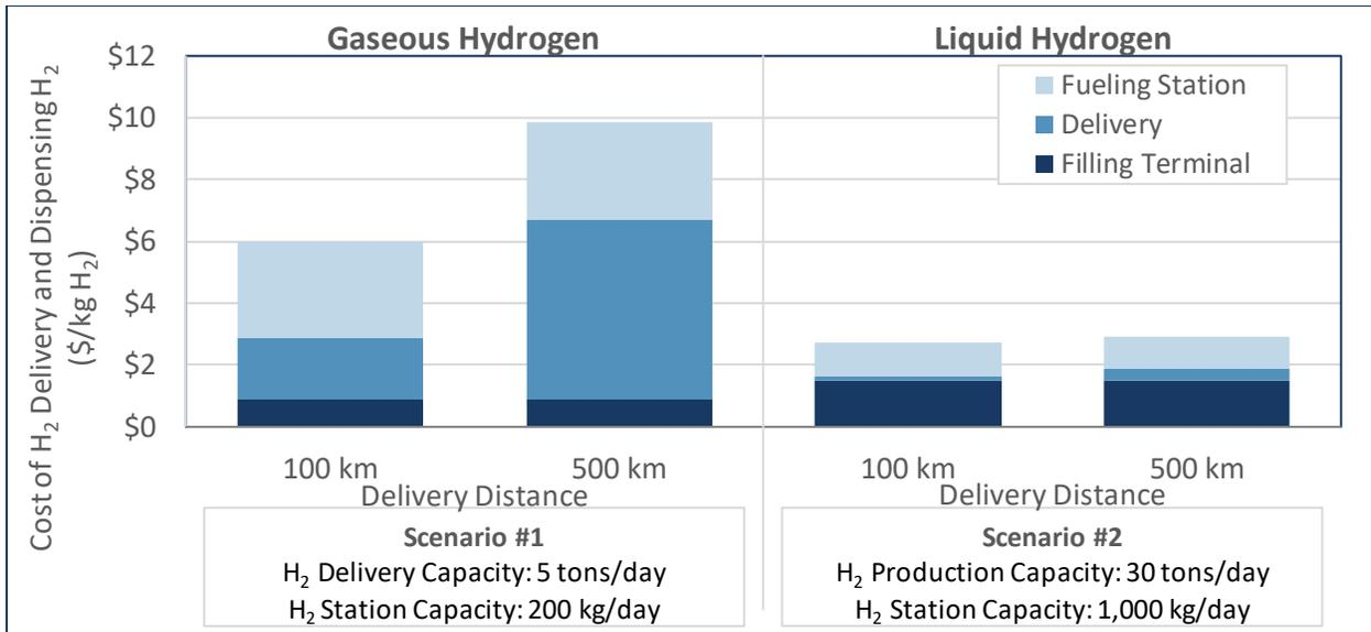
**Figure 18 – Truck-Based Delivery Cost for Hydrogen as a Compressed Gas and Cryogenic Liquid<sup>1</sup>**
