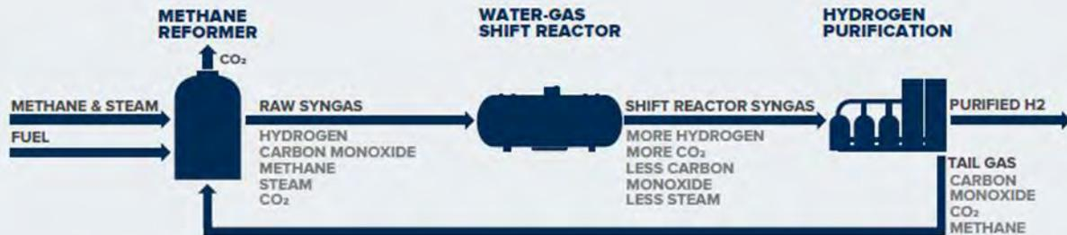
Figure 14 – Steam Methane Reforming (SMR) Process and Description<sup>1</sup>
