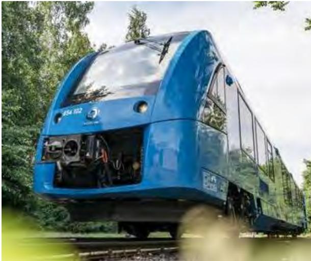
**Figure 26** – Alstom Hydrail with Hydrogenics Engine (Photo courtesy of Alstom)<sup>2</sup>
