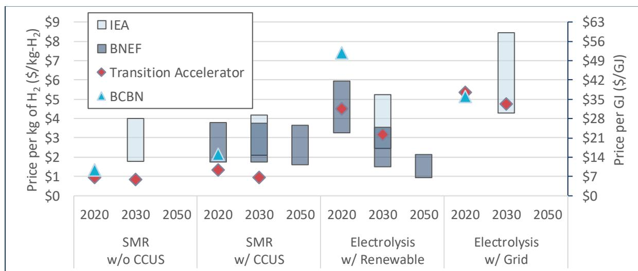
**Figure 16** – Comparison of Hydrogen Production Pathway Costs 2020, 2030, and 2050<sup>1,2,3,4</sup>
