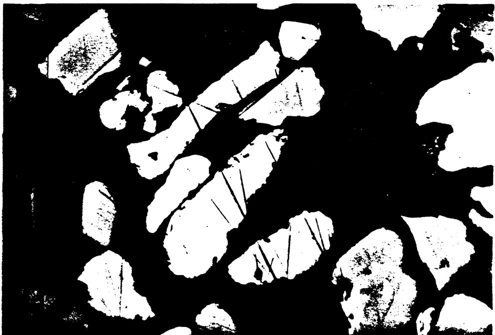
Fig.19. Photomicrograph showing anhedral-subhedral gold grains. Varying Ag-content is reflected by the colour differences. Native bismuth and bismuthinite occur as well. Oil immersion. Bar scale 0.1 mm.
