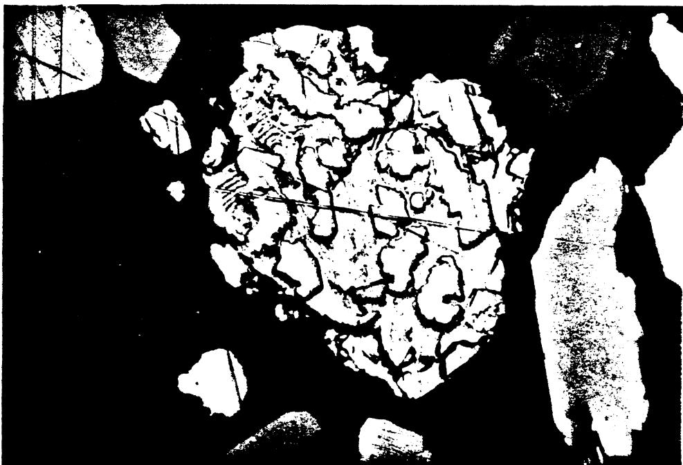
Fig.20. Photomicrograph showing myrmekitic intergrowth between native gold and native bismuth. Oil immersion. Largest dimension of grain - 0.3 mm.
