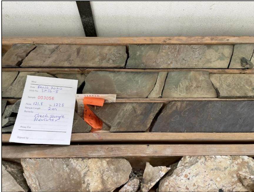
**Figure 7-4: Core Photo of Moody Hill Central Drill Hole SF16-08 (120 to 132 m) with Green Grey Lithologies and Manganese-Iron Mineralization**
