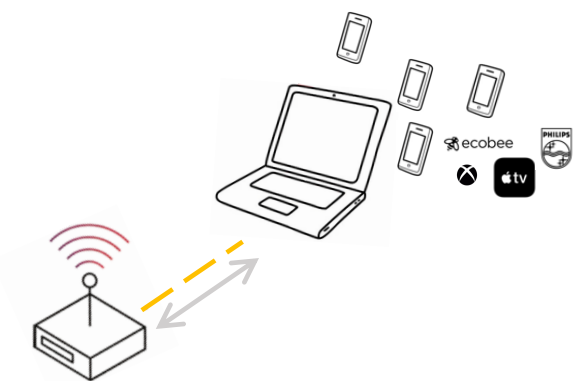
Figure 1: Legacy Wi-Fi offers a single channel, shared by all devices
