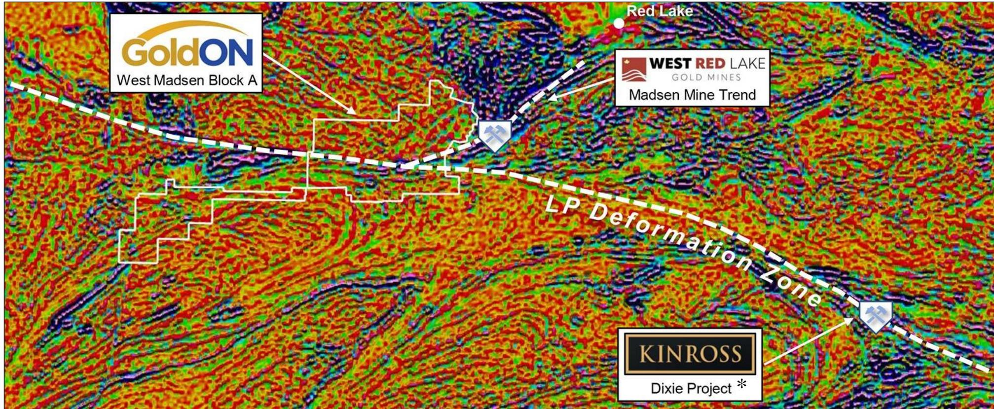
The Dixie Project is also located within a magnetic low along the LP deformation zone/fault. The regional second vertical derivative magnetic signature suggests that this important deep-seated gold-bearing structure could be traced northwesterly through GoldON's Block A claim group where several prominent magnetic lows are coincidentally located.
