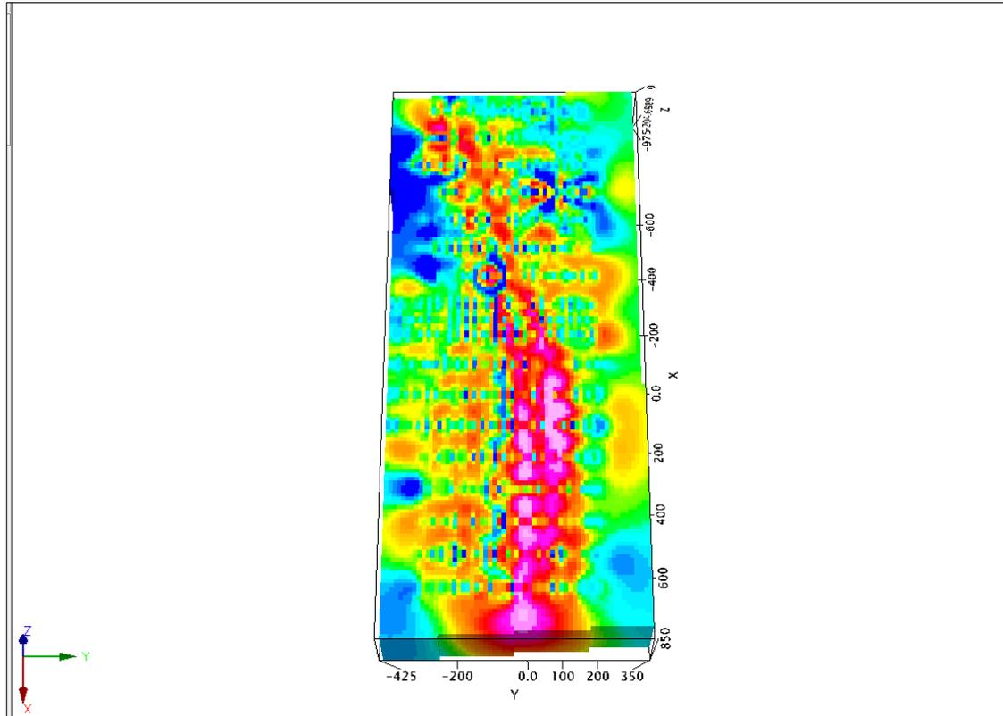
Figure 37: 3D GeoSoft Voxel of Inverted Chargeability Data Looking north
