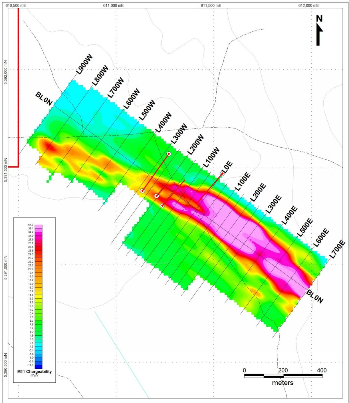
Figure 36. Altius IP Chargeability Survey with Drill Locations (n=2)
