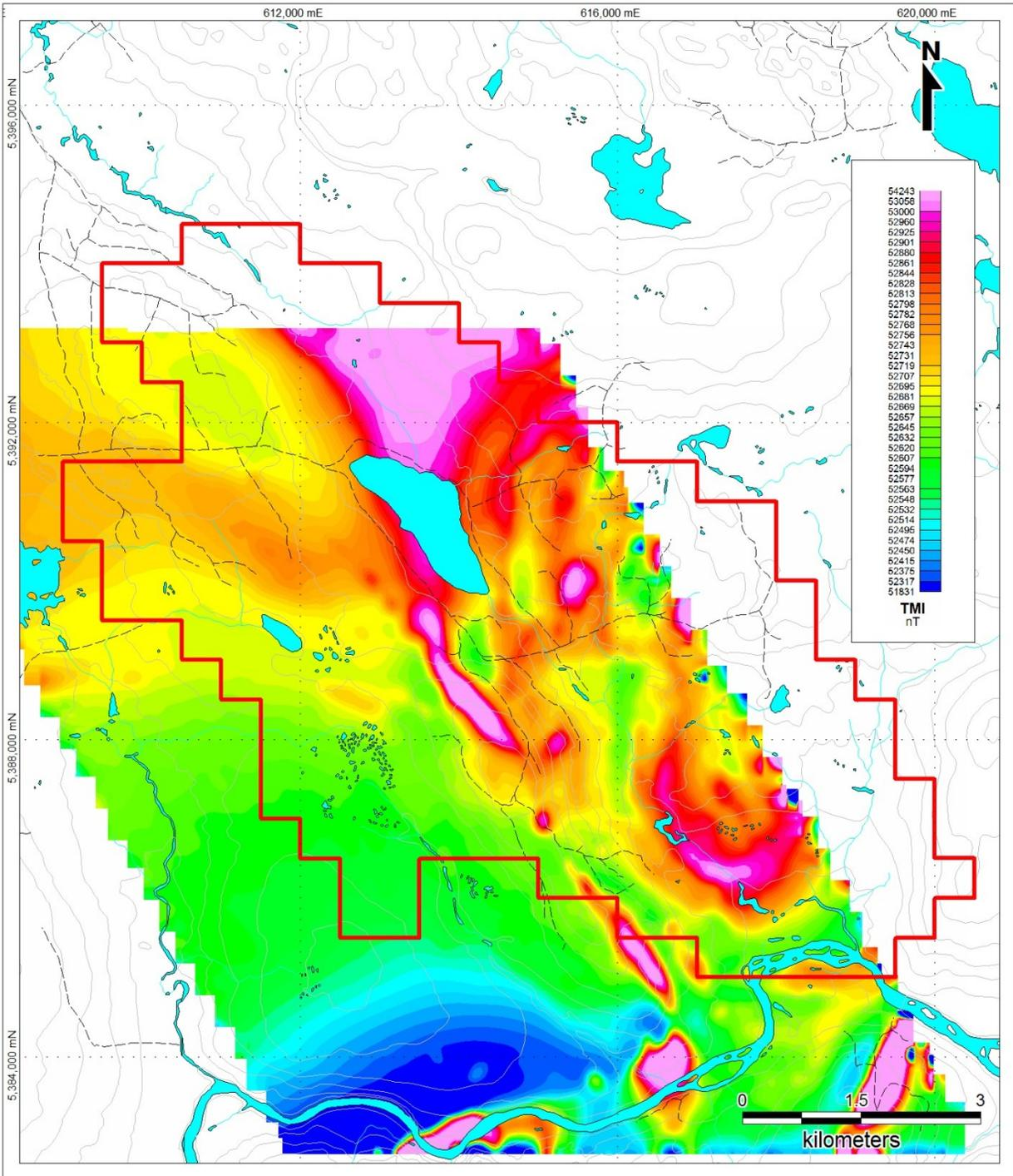
Figure 27: Altius/Goldak Airborne Total Field Intensity Magnetics (TMI) Map
